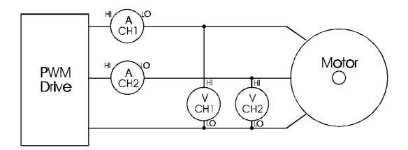
This leaves one channel free for example to make the measurement on the DC Bus.
