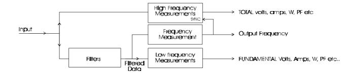
This technique allows both high frequency and low frequency data to be obtained from the same samples, and allows the high frequency measurements the be synchronised to the low frequency signal.
