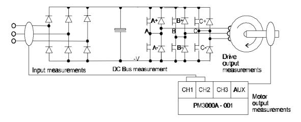
Measure Input power Measure Mechanical Power
