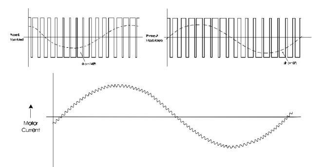
The output voltage from a PWM drive the complex waveforms shown below:
